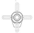
Note that the tether can be mounted in four different orientations.
