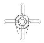
Note that the tether can be mounted in four different orientations.
