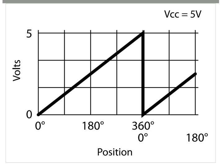
Analog output is only available in 10-bit resolution. The analog output voltage is ratiometric to the power supply voltage and will typically swing within 15 millivolts of the power supply rails with no output load. This non-linearity near the rails increases with increasing output loads. For this reason, the output load impedance should be  $\ge 4.7 k\Omega$  and less than 100pF. The graphs below show the typical output levels for various output loads when powered by a 5V supply.
