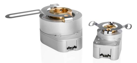
▲ Hollow Bore Encoders have internal bearings and a shaft with a hollow bore. The hollow shaft mounts over the motor's shaft or another shaft in the system. A flexible tether is used for mounting.
