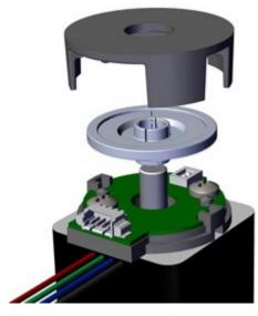
**Step 4: Cover Installation**Snap cover onto base.
