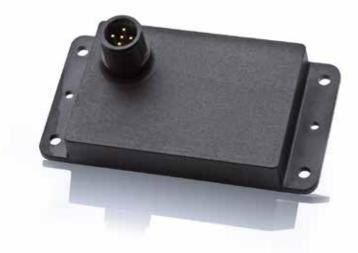
The T7 Absolute Inclinometer from US Digital® represents a breakthrough in high-accuracy, sensor technology for solar tracking systems and CSP and CPV applications. Providing the capacity to accurately sense tilt angles over a full 360° range in a single axis, the T7 incorporates a resolution of 0.01° and is accurate to 0.1° in temperatures ranging from 0°C to 70°C.
