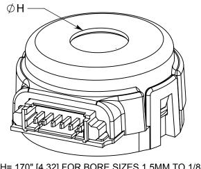
H=.170" [4.32] FOR BORE SIZES 1.5MM TO 1/8" H=.295" [7.49] FOR BORE SIZES 5/32" TO 1/4"
