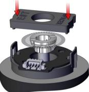
Mounting Screws: 2-3 in-lbs torque
