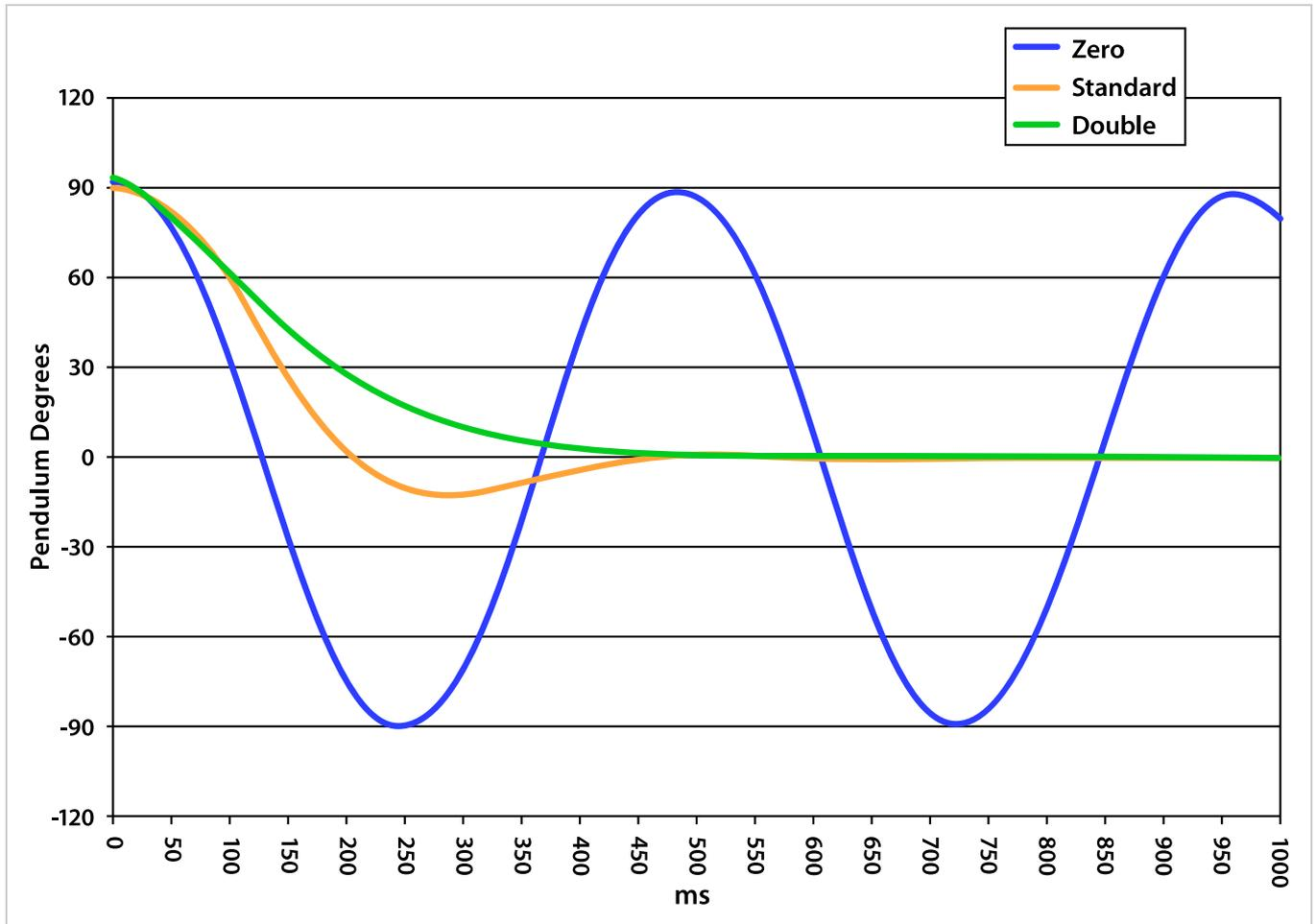
Damping affects settling time and overshoot. Standard damping will fit most applications. Double damping eliminates oscillation but settles to the final position more slowly. Some applications may require double damping to average out cyclic motion such as found in moving vehicles. Damping options can be specified when ordering.
