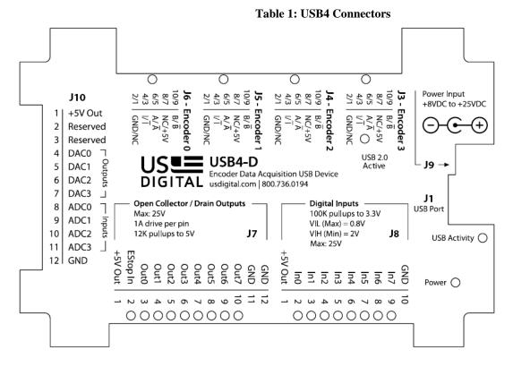
**Figure 1 Connector Layout**
