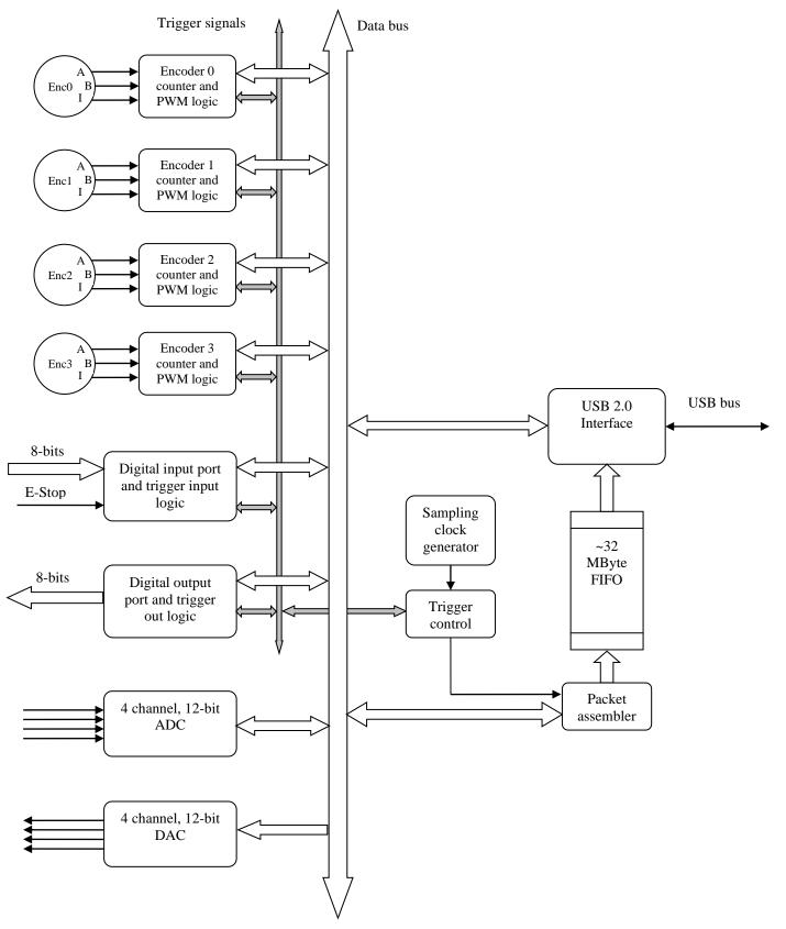
Figure 2: USB4 Block diagram
