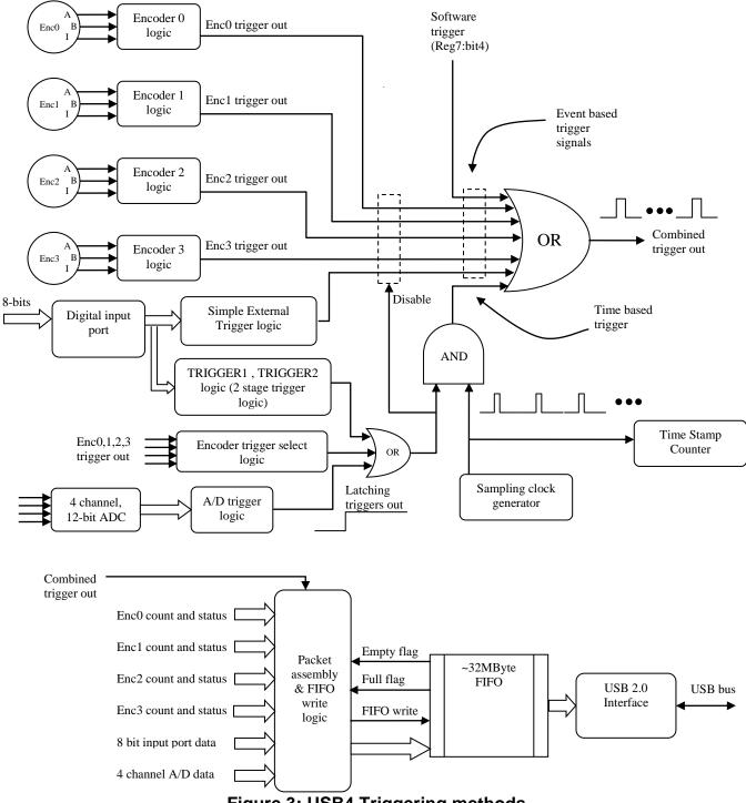
Figure 3: USB4 Triggering methods
