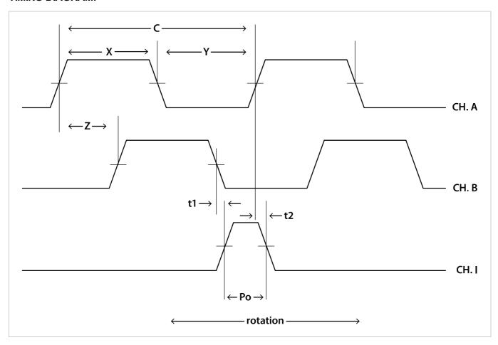
CPR: The number of Cycles (C) of the A or B outputs Per Revolution.
