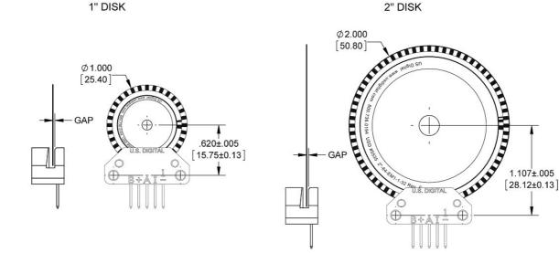
RECOMMENDED DISK GAP:  $.020^{+.005}_{-.010}$  [0.51 $^{+0.13}_{-0.25}$ ] (.020 $^{\pm}$ .005 [0.51 $^{\pm}$ 0.13] FOR 32 CPR 1" DISKS OR 64 CPR 2" DISKS)
