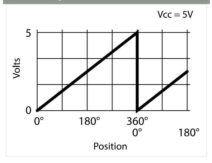
Analog output has 12-bit resolution. The analog output voltage is ratiometric to the power supply voltage, which is typically 5.0V
