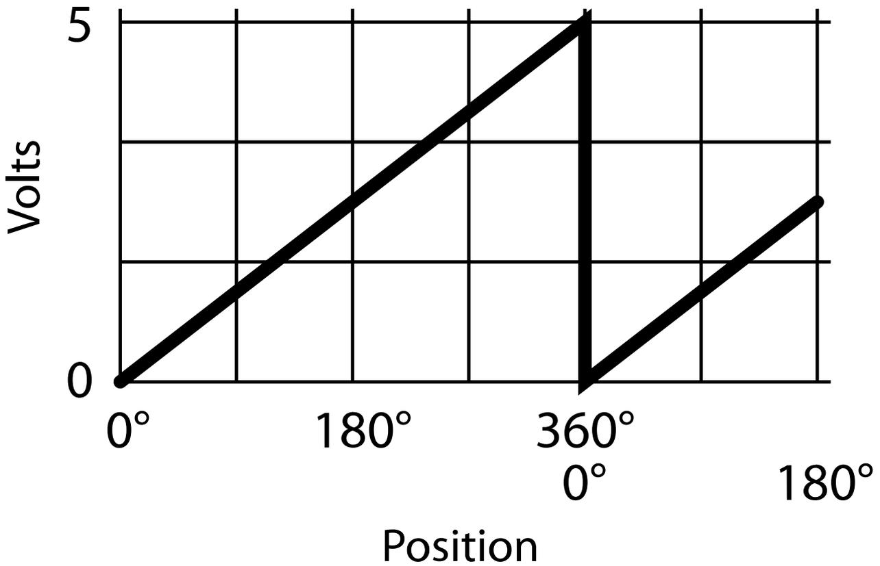
Analog output has 12-bit resolution. The analog output voltage is ratiometric to the power supply voltage, which is typically 5.0V
