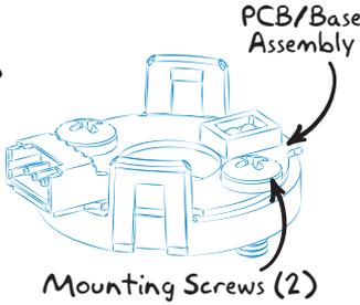
Attach the "PCB/Base Assembly" to the AndyMark Toughbox (not shown) using the pre-installed mounting screws.
