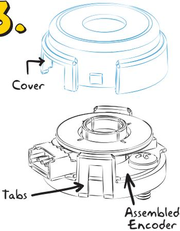
Snap the cover onto the assembled Encoder Base. Press in on the tabs to ensure that the cover fully latches.
