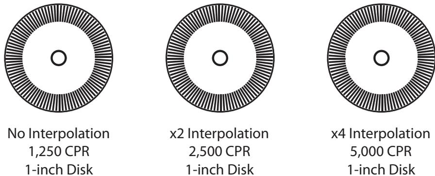
The drawing shows a 1-inch disk with 1,250 lines (1,250 CPR). Through the technique of electronic interpolation (signal processing that takes place within the encoder itself), the CPR can be increased to 2,500 CPR using x2 interpolation; and to 5,000 CPR using x4 interpolation.
