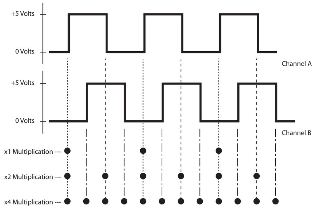
This is called *resolution multiplication*. System designers can implement it by using an encoder to counter interface chip such as an LS7183N.
