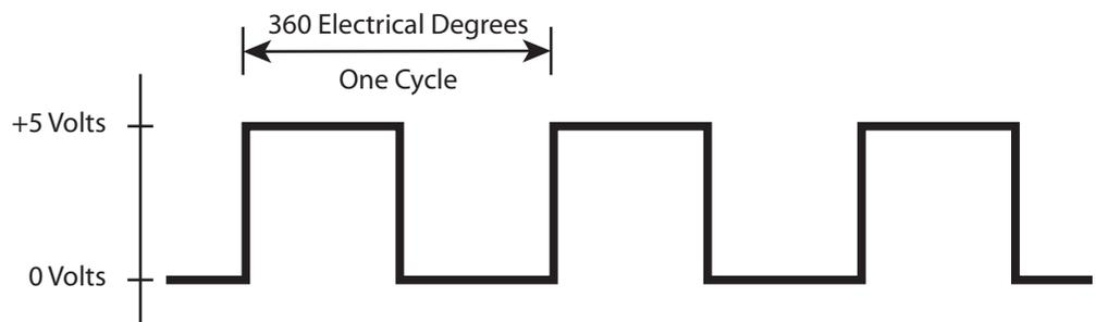
Resolution, when applied to optical encoders, specifies the number of times the output signal goes high per revolution. This number can match the number of lines on a disk; or, especially with higher resolutions, it can be a multiple of the number of lines. (We'll talk about this more in the section on *Scalability*, below.)
