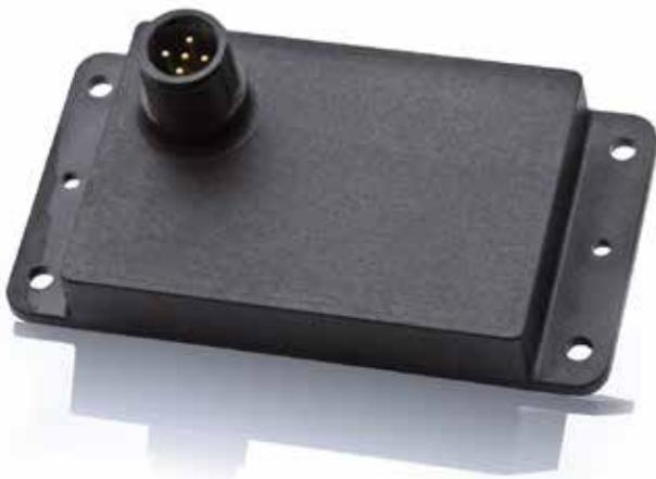
The T7 Absolute Inclinometer from US Digital® represents a breakthrough in high-accuracy, sensor technology for solar tracking systems and CSP and CPV applications. Providing the capacity to accurately sense tilt angles over a full 360° range in a single axis, the T7 incorporates a resolution of 0.01° and is accurate to 0.1° in temperatures ranging from 0°C to 70°C.
